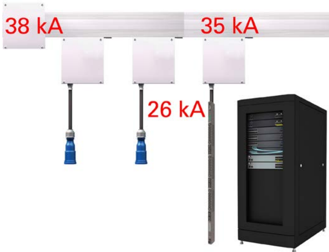
Figure 8.1.2.b Typical data center busway, busway drop units and rack PDU with high fault current levels.
