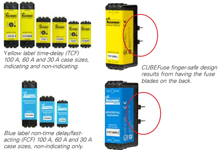
Figure 8.1.8.1.a Time-delay (TCF) and fast-acting (FCF) CUBEFuse.
