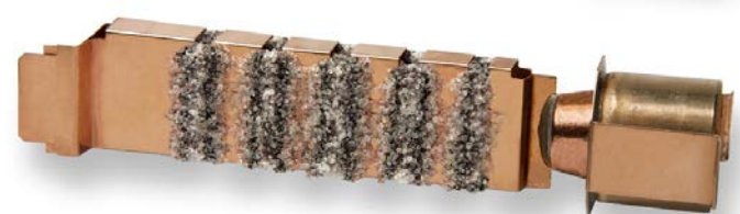
Figure 3.1.3.2.e Arc-quenching filler material helps suppress the arcing by melting and forming folgurite.
