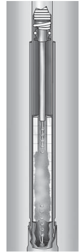
Vapor quenches arc at first current zero
