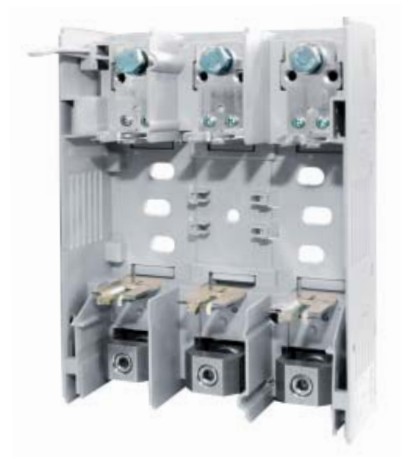
EBH1 for installation on mounting plate, picture of fuse switch disconnecter without fuse links cover and terminal shrouds, top cable terminal - M screws, bottom cable terminal - V-clamps, (EBH1 bottom cable terminal - M screws, top cable terminal - V-clamps)
