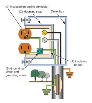
For protection against both voltage spikes and electronic noise, choose an isolated ground surge protection receptacle.
